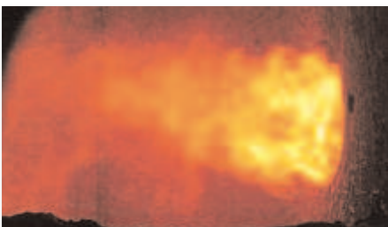
Figure 6. This image shows a flame that is pulled back into the throat (high swirl). This can lead to thermal destruction of the burner (image copyright IFRF)
