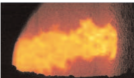
Figure 7. This image shows a long loose flame (low swirl), which is not properly anchored and can be unstable (image copyright IFRF)
